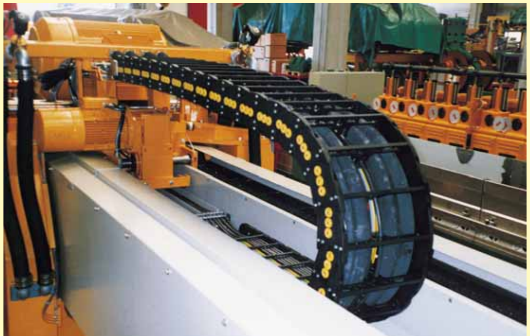
Nylon chain, type SR310, in a self-supporting state.
